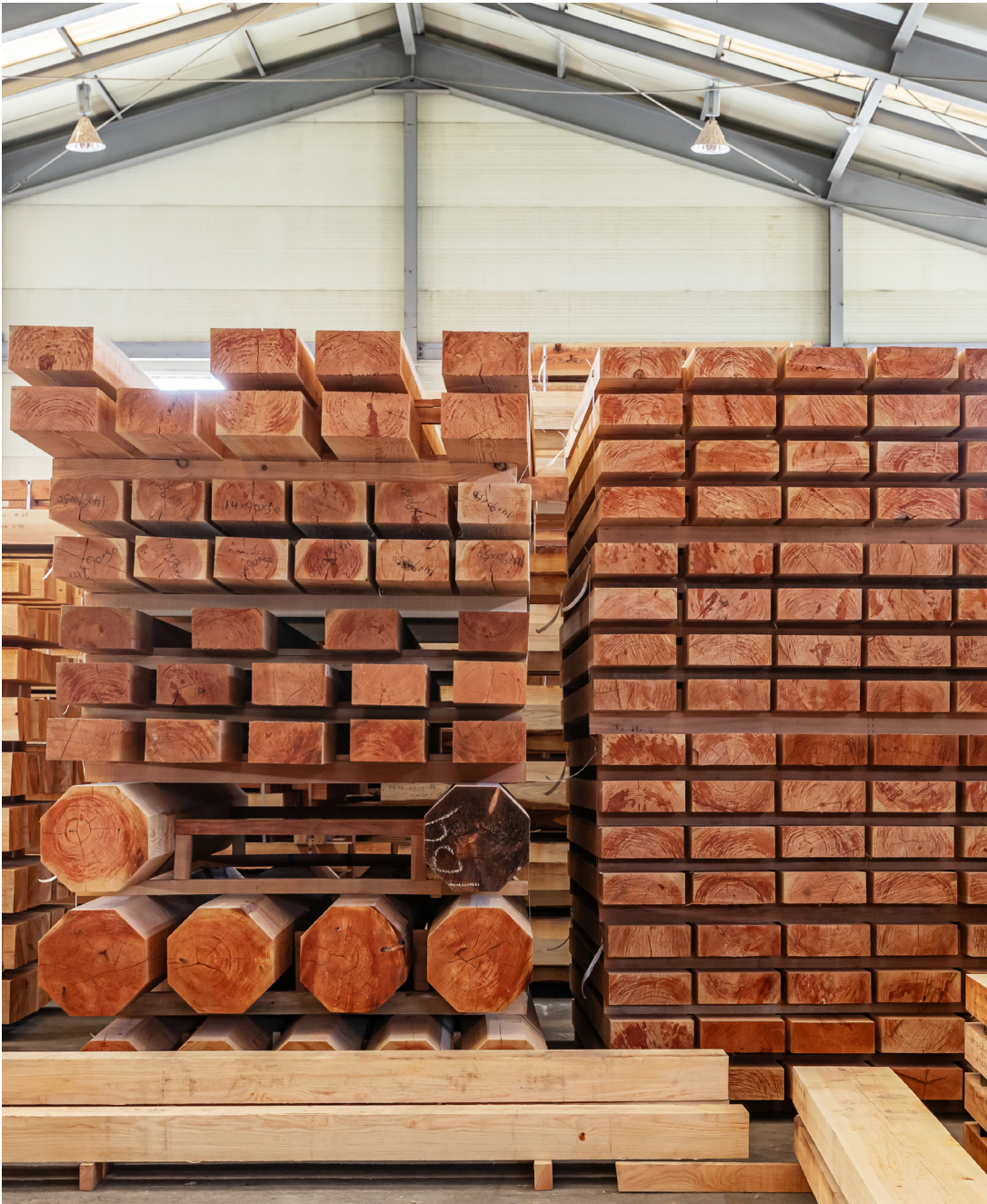
Donghae City Timber Storage Depot: Natural drying in progress
